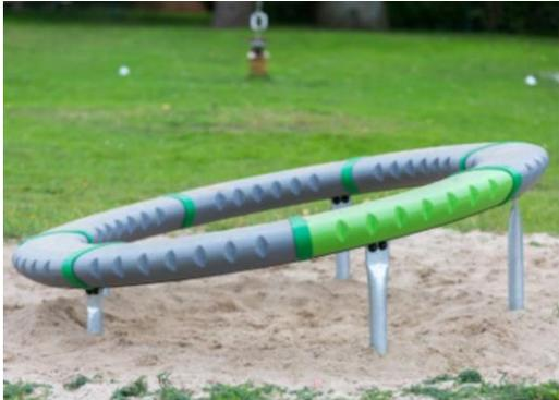
The Supernova is a unique carousel with no center point placed in an angle of 10° which makes it turn when children walk the ring. The outside ring diameter is 208cm and the upper point is 60cm above ground level.
