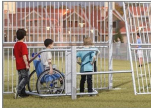
The wheelchair entrance is constructed of 80 x 80 x 3mm post with Ø 48mm tube and 2 stainless steel 16mm hinges. The opening is 95cm wide and 112cm long, this will allow people in a wheelchair to enter the MUGA but stops mopeds and motors.
