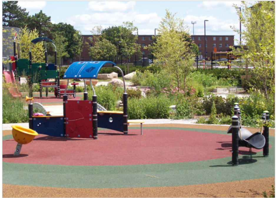
At both ends of the arched bridge are formal play areas comprised of KOMPAN play equipment on poured-in-place safety surfacing of complementing primary colors.
